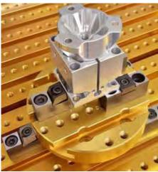
material cost. These modular clamps and stops are ground to the same height as our Large Modular Pitbull<sup>®</sup> Clamp (page 13) providing even greater versatility.
